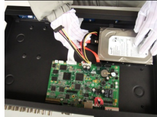
5. Connect the data wire
