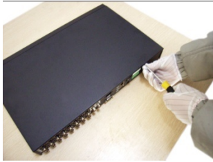
1. Loosen the cover screw
